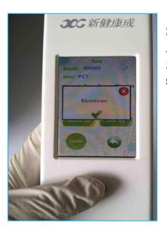
Step 6: Shut down After the test, press and hold the power key (about 5 seconds) to pop up the shutdown prompt box and select " $\sqrt{}$ " to shut down.
